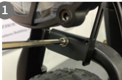
1. Put the headlight on the arch of the fork. Locate the bolt hole.
