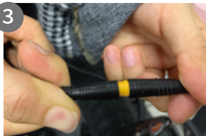
3. Connect the yellow headlight cable. (Pay attention to the Arrow mark on the cable). Click this link to watch cable connection video: https://youtu.be/WOrH8cbQgQk
