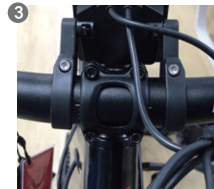
3. Center the handlebar and adjust the direction, make sure the handlebar is centered on the stem.
