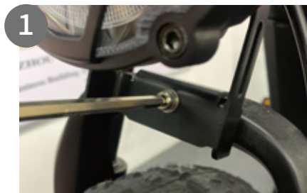
1. Put the headlight on the arch of the fork. Locate the bolt hole.
